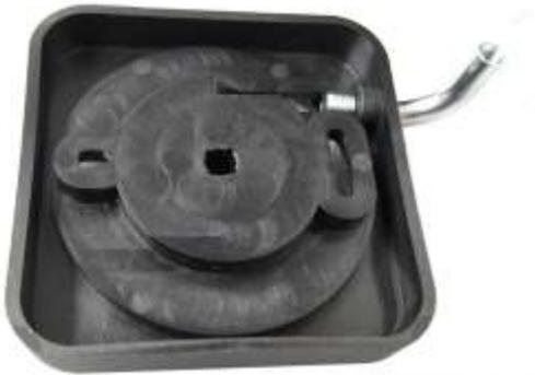
Insert the steel cable inside the bend pipe as shown in the figure.
