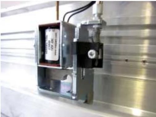
When the knob is in the released position, the electric lock must remain open and free the leaves.
