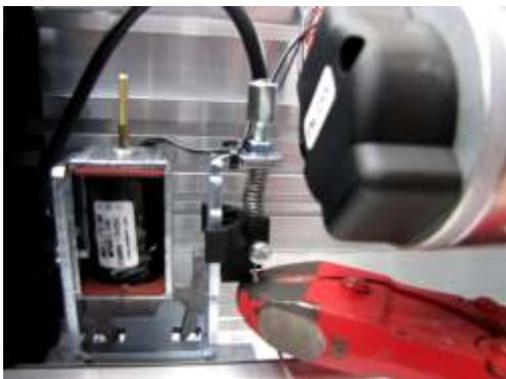
Cut the exceeding steel cable from the release anchor.
