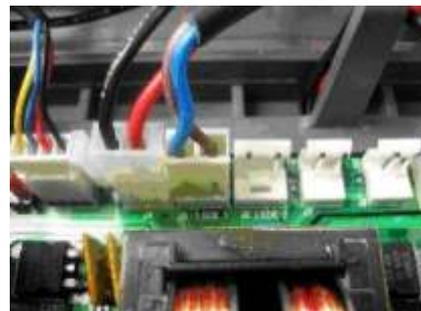
The electric lock kit includes a power supply cable. This cable has two wires on one end that are connected to the electric lock solenoid wires with the specific terminals. The other end of the cable has a connection that is inserted in the LOCK1 connector on the Evolus operator electronic control unit.
