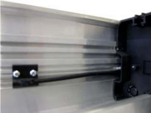
Insert the sheath and the metal cable inside the plastic component.
