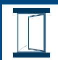
CASEMENT FRAME hinges in a vertical side, inside opening, actuator mounted inside.
