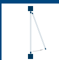
OUTWARD FRAME hinges in the top side, outside opening, actuator mounted inside in the bottom.
