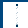
LOUVERS FRAME rotation of louvers in medium side position, opening with a control lever.
