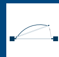
DOMES AND SKYLIGHTS hinges in a side, opposite outside opening, actuator mounted inside.
