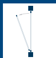
VASISTAS FRAME hinges in the bottom side, inside opening, actuator mounted inside in the top.
